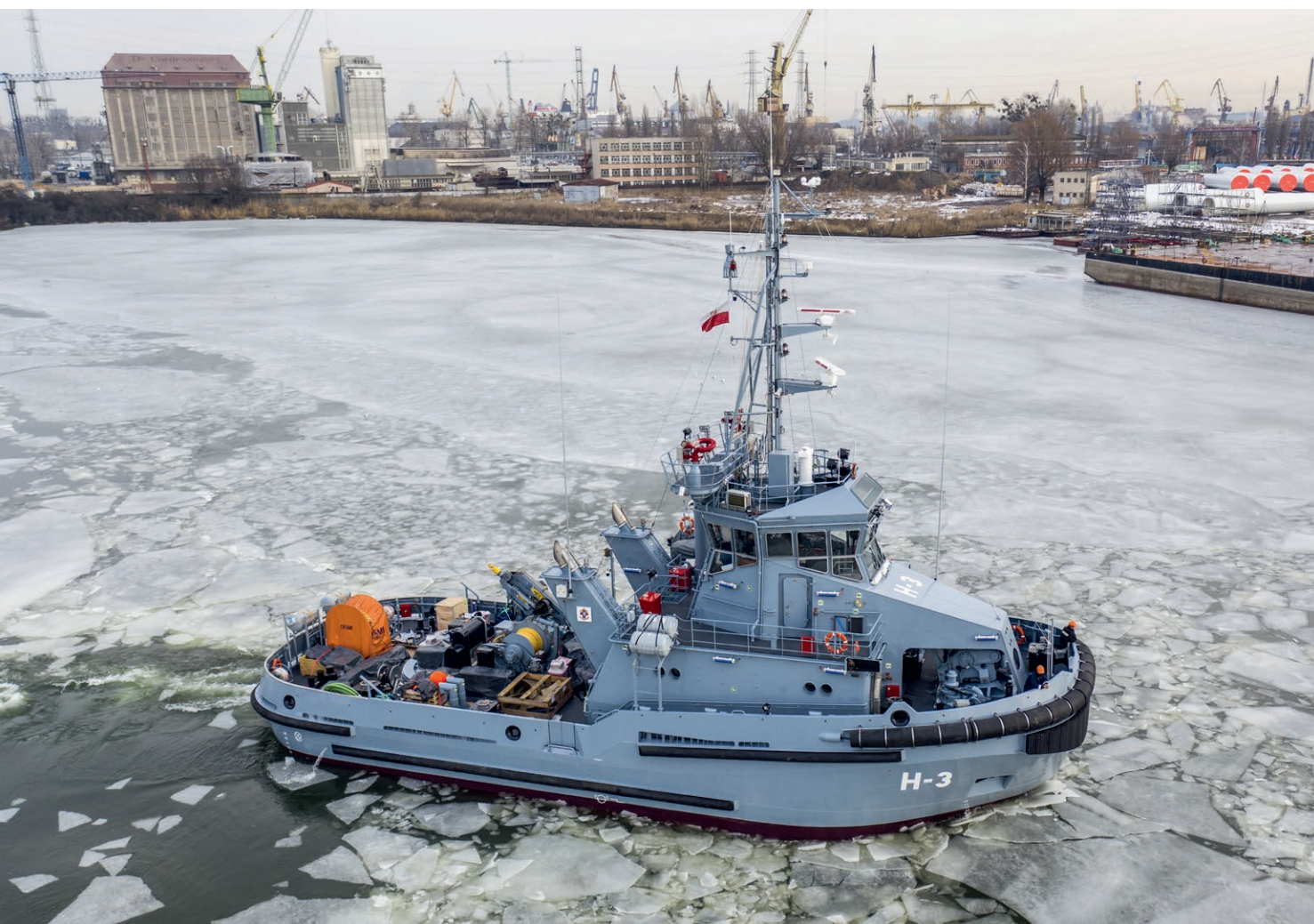
H-3 Leszko . The ice class of the tugs allows them to operate in heavy ice conditions
