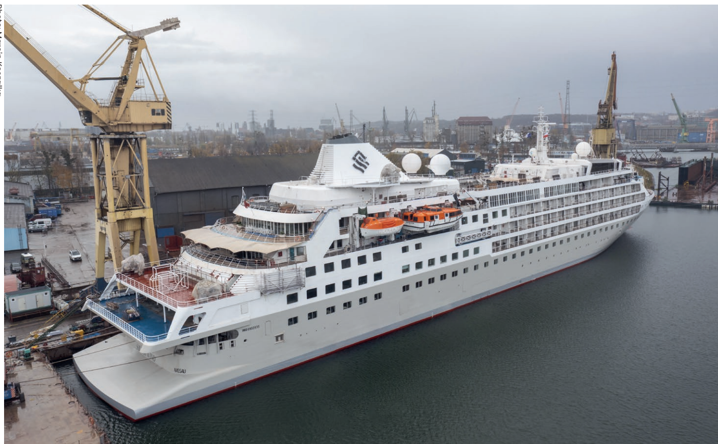
At the stern, Remontowa installed a duck tail extension weighing 150 tonnes
