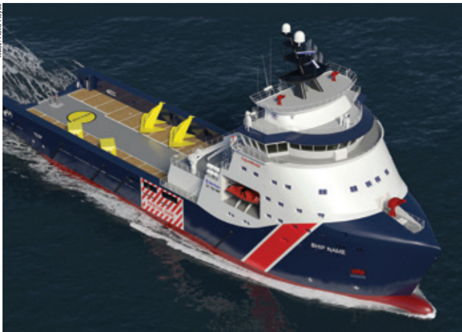
The Rolls-Royce Wave Piercing hull will cut through the waves, minimizing the green water intake and ensure a safer and more comfortable journey.
